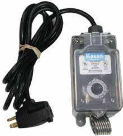
The C-10 Thermostat Controller is an inexpensive way to control the operation of your Kasco De-icer by using air temperature. The C-10 plugs into a standard 120V outlet and allows you to set an air temperature setting to turn the de-icer on when the temperature drops below that setting, allowing you to save money on electrical bills.
