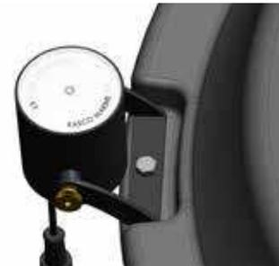
5. Install the 1/4" Flat Washer, 1/4" Lock Washer and 1/4" Nut against the underside of the float tab as shown in Figure 5. Tighten the nut until snug using the 7/16" Wrench.
