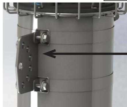
Warning! Be sure flat surface of plate is facing to the right of the unit as shown. Failure to do so could result in the loosening or unthreading of the pipe fittings while in operation.
