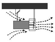
During unit operation, water is circulated from 360° around the unit. The Circulator draws in water and circulates it throughout the pond.
