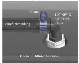
8. Install strain relief over tubing and secure to diffuser base as shown using 7/16" socket and wrench. A properly installed strain relief will prevent any damage to the diffuser assembly when it is lowered in the water or pulled up at a later date for maintenance.
