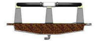
4. Install vent plug once base is completely full.
