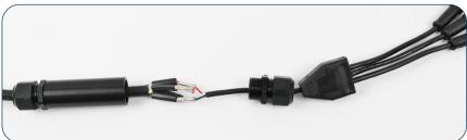
8. Slide the shrink tube over the connectors so it covers all the exposed wires and crimp connections. Heat the shrink tubing until it is tight around the connections.
