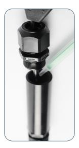
11. Screw in the small gland cord grip (splitter side) into the cable joiner completely and tighten cord grip nut to splitter cord making sure no wires are exposed on either side of the cable joiner assembly. Let it sit for 30 minutes while the potting cures.
