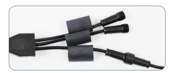
14. Connect the fixture connectors to the splitter connectors. Slide the nut from the fixture half of the connector over until it engages the threads on the splitter half of the connector. Turn clockwise to secure the two halves snugly together. (Note: Over-tightening may damage components)
