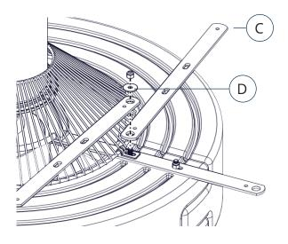
2. Repeat for the other two sides of the unit, overlapping the free ends of the brackets and aligning the holes. Tighten the 3/8" nuts until secure.
