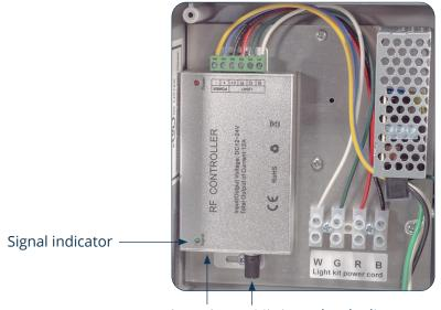
Connect light kit power cord wires to this terminal block.
