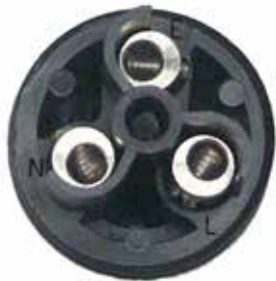
Figure 5: Wire Connections Brown wire to terminal L Blue wire to terminal N Green/Yellow wire to terminal E
