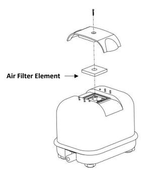
Replacement air filter elements are readily available. Contact your local Kasco distributor and ask for the appropriate Replacement Air Filter Element per the list below.
