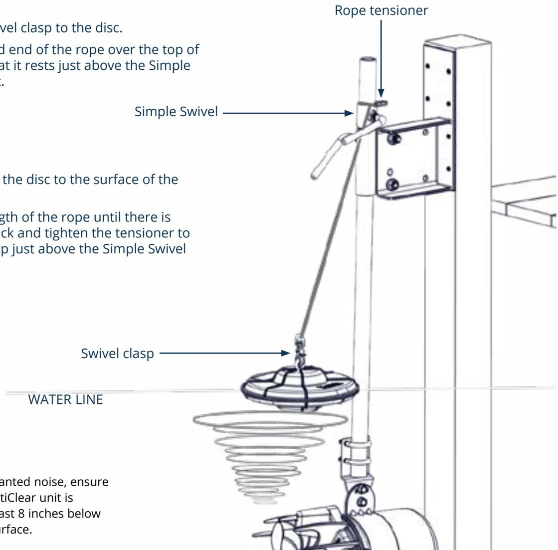
**NOTE** To avoid unwanted noise, ensure that the AquatiClear unit is installed at least 8 inches below the water's surface.
