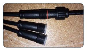
7. Slide the Nut from the Fixture half of the connector over until it engages the threads on the Cord Splitter half of the connector. Turn clockwise to secure the two halves snugly together. (Note: over-tightening may damage components.)
