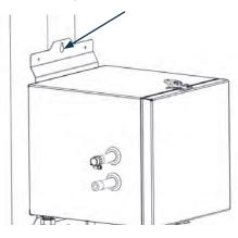
Predrill a 5/32" hole on the marked location. Insert a lag screw. Do not fully tighten.
