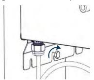
Tighten the top lag screw until the bracket is secure to the post.
