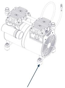
NOTE Remove vibration mounts for 1/2HP compressors going into the new style small cabinet.
