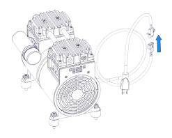
Remove the push-to-connect fittings and plugs from the old compressor. Thread them into the new compressor as shown.
