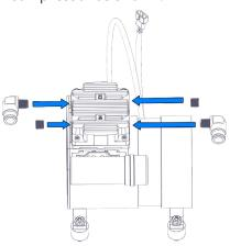
Remove vibration mounts from the new compressor. These are not needed for the new style RA1-3 cabinets.
