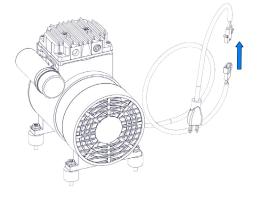
Remove the push-to-connect fittings and plugs from the old compressor. Thread them into the new compressor as shown.
