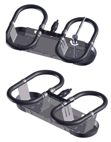
9. Slide the provided hose clamp of the appropriate size onto the SureSink™ Tubing. Feed the weighted tubing over the substrate connector, leaving plenty of slack. Make a generous loop and secure the tubing to the barb fitting with the hose clamp. Tighten down the clamp with a flathead screwdriver or a 1/4" nut driver.
