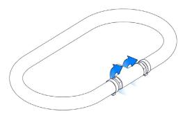
2. Assemble both tubing assemblies to the inlet check valve assembly.
