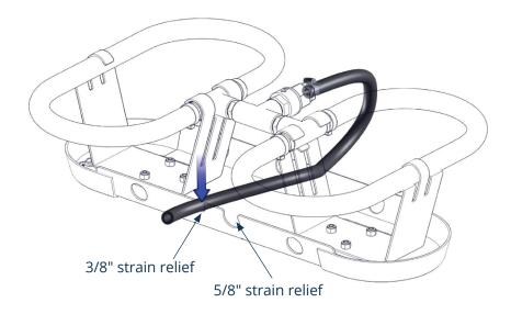
11. On the other side of the connector plate, press the weighted tubing into the remaining strain relief notch of the same size (diagonal from the notch on the opposite side of the plate). Ensure that the SureSink™ Tubing snaps into place in both correctly sized notches before installing the unit.
