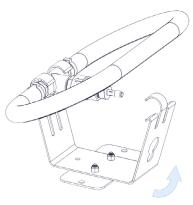
Firmly press the SureSink tubing into the narrower part of the keyhole to create a strain relief for the diffuser.
