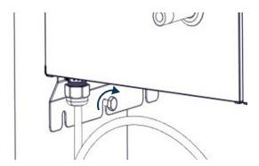
Predrill a 5/32" hole on the marked location. Insert a lag screw. Do not fully tighten.
