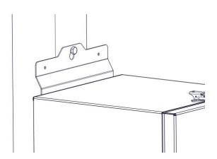
Tighten the top lag screw until the bracket is secure to the post.
