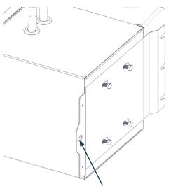
The single mounting hole on the bracket should be on the opposite side of the power cord.
