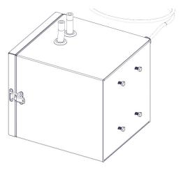
Slide the bracket until the bolt heads are interlocked with the narrow grooves. Tighten bolts with 7/16" socket or wrench.
