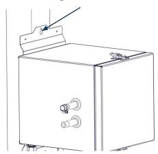
Predrill a second 5/32" hole in the center of the middle notch on the bottom of the bracket. Insert the next lag screw and tighten until the bracket is secure to the post.
