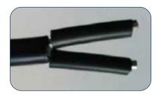
5. Slide one shrink tube over the white wire and one over the black wire.
