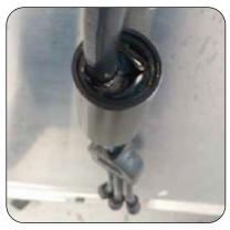
10. Hang the cord in a vertical position with the open end of the cable joiner (splitter side) on top. Use the potting kit to fill the inside of the cable joiner, making sure the potting completely covers the black jacket of the splitter cord.
