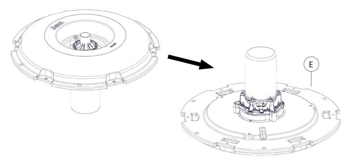
4. Position the power cord in the dedicated cord channel. Slide the bottom screen (J) over the unit's motor housing (H) and rest on the bottom side of the float.
