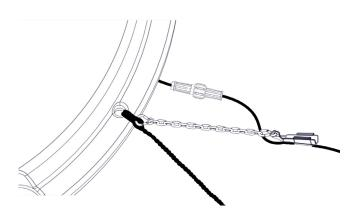
Providing strain relief on the cord helps ensure that its weight and any strain placed on it in the water will not cause the float to tilt or cause damage to the unit.
