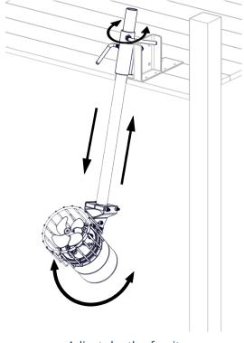
Adjust depth of unit and angle of operation.
